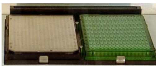
Figure 2 Simultaneous Collection on MALDI Plate and Microtiter Plate
