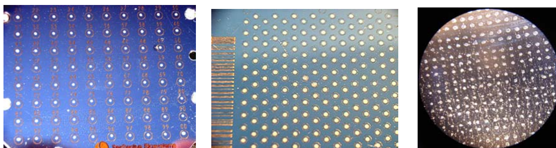
Figure 1 Spotting Precision for difficult Targets with 100 spots, 192 spots and even with 5625 Spots on only 5 x 5 cm (2x2 inch) area
