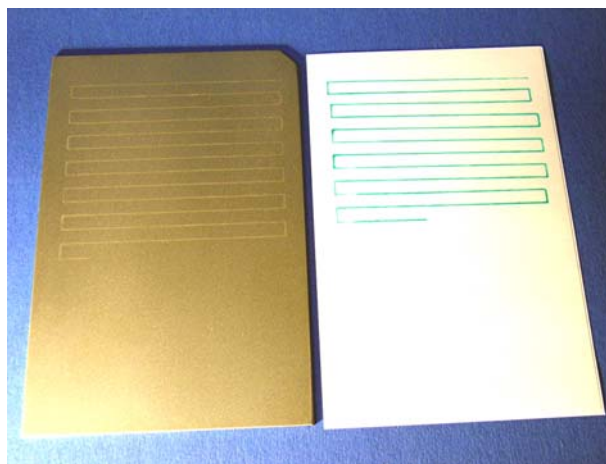
Figure 6 Continuous collecting of eluates in lines instead of discrete spots
